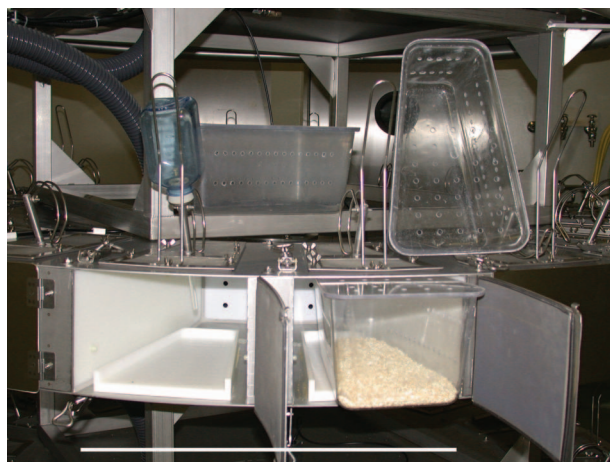
Figure 2. UMTS exposure device with two opened exposure segments. Note the specifically constructed trapezoidal polycarbonate cages with several ventilation holes. Water supply was assured by the externally mounted water bottle and a drinking nipple made of glass penetrating into the cage through a tube dimensioned as 'waveguide beyond cut-off', scale bar 50 cm.
