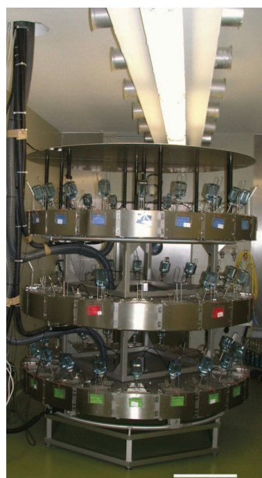
Figure 3. Three-decker UMTS exposure device for mice. Scale bar 50 cm.
