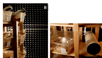
Fig. 1. BI study on 1.8 GHz base station RFR: exposure system. The rat cages were located in wooden circular-shaped devices, as in a sort of condominium. Each single exposure device served at least 400 rats (A). The exposure rooms were totally shielded in order to minimize the effect of field non-uniformity due to reflection and consequent interference caused by the walls (B). Detail of the RF feedback probe used to measure the field (TSP02001 field sensor) and of the animal cage with methacrylate markers, cover and mangers (C).
